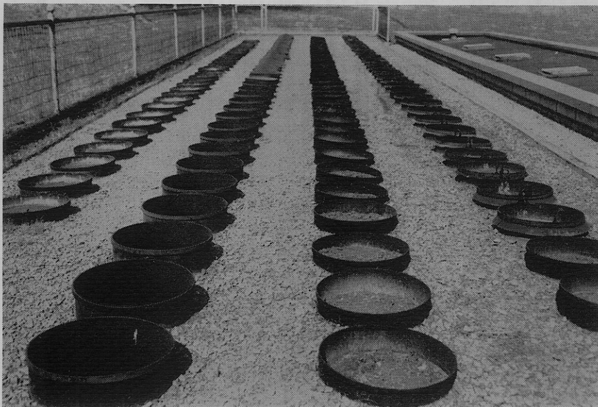
Figure 1. Installation of lysimeters Rain-water drainages pass into building at right
